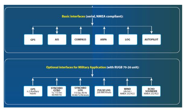
Figure 2. Connection of ECDIS
